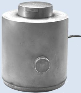
Typical compression-type load cell
