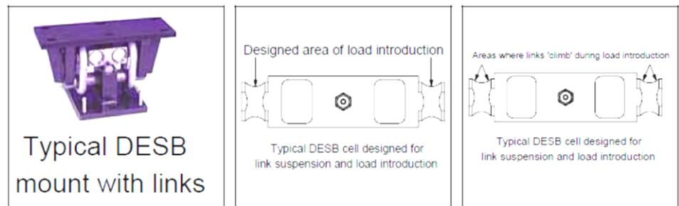
2. In another form the load cell is bolted at the ends and the load is introduced in the center by means of a link. This embodiment suffers greatly because the load cells natural physical tendency to shorten during loading is prevented by the mounting bolts. This causes serious hysteresis\* errors. This affects the accuracy and performance of the scale and the end user suffers from the results of an inaccurate scale. \* Defined in sidebar.
