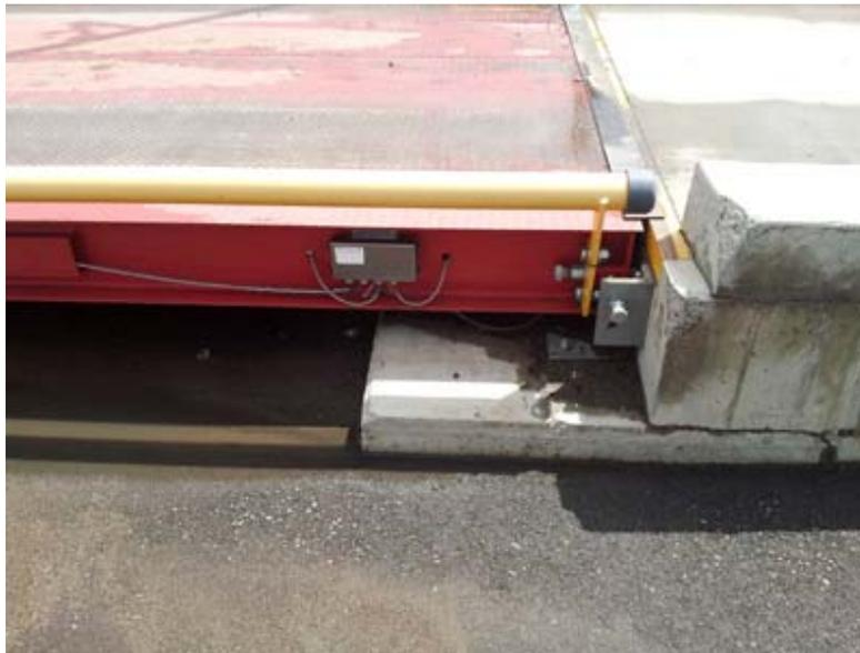
equipped with Intalogix<sup>®</sup>, a technology that digitizes analog load cell signals to achieve a high level of lightning/surge protection and enhance the speed of weighing communications. **Figure 3** shows a truck scale, equipped with Intalogix<sup>®</sup> working efficiently to meet the needs of Steel Etc.
